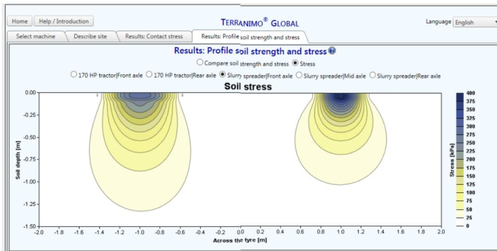
Figure 10. Terranimo-predicted stress distribution in the soil profile below a similarly loaded and inflated implement tyre at field capacity water content (left) and at the wilting point (right).
