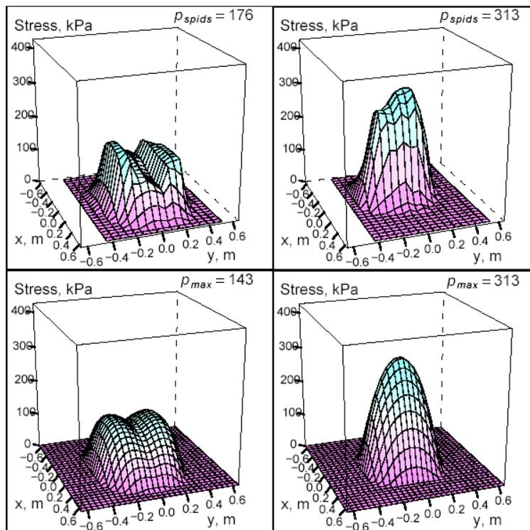
Figure 8. Measured vertical stress at the tyre-soil interface (upper part-Figures) and FRIDA-modelled stress-distribution (lower-part Figures). The data derives from a Michelin Cargobib 650/65R30.5 implement tyre loaded with ~60 kN (~6 tonnes) and either the recommended 1.0 bar (left) or 2.4 bar (right) inflation pressure. Data from Schjønning et al. (2006).
