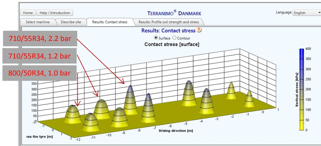
Figure 5. The contact area stress.
