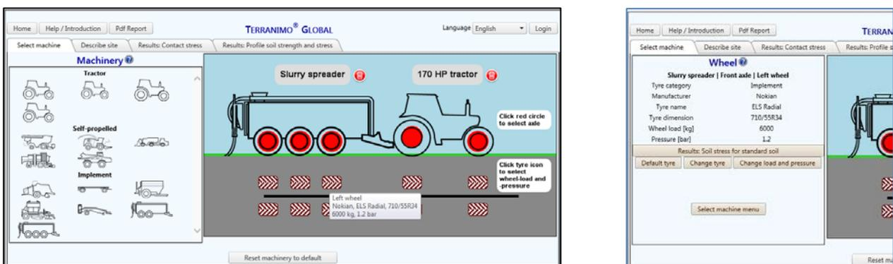
Figure 2. Tyre type, wheel load and tyre inflation pressure is shown for wheels on the machinery if placing the cursor on top of the tyre icons (left). If clicking the icons, a menu opens, enabling change of tyre and modifications in wheel load and inflation pressure for the selected tyre (right).
