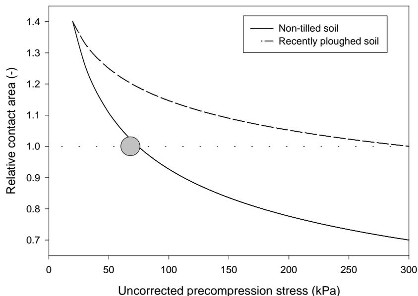
Figure 9. Terranimo® prediction of topsoil strength effects on the tyre-soil contact area. The gray symbol represents the topsoil strength condition for the comprehensive data set (Schjønning et al., 2006) being the main data behind the equations for estimating FRIDA parameters in Terranimo® (Schjønning et al., 2015b).
