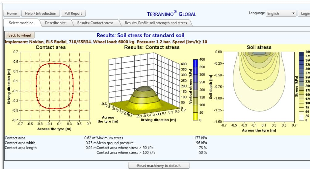
Figure 3. A special facility allows for studying the performance of a selected tyre at the selected wheel load and inflation pressure. Importantly, this specific graphics relate to ‘standard’ soil conditions, which in Terranimo® is defined as a sandy soil at field capacity water conditions.
